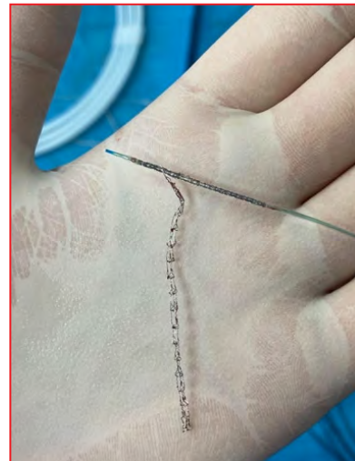
Figure 3. Picture of the extracted stent with deformed stent.
